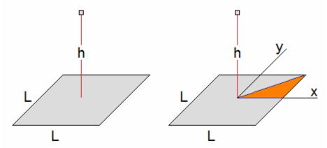
We could integrate over the entire square or, to simplify the calculation just consider one triangle (as shown above) and multiply by 8.
