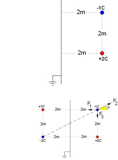
a) The net electric force on the negative point charge. We replace the infinite plane with two mirror image charges as shown above. Then, to find the force on the negative charge we consider three forces:
