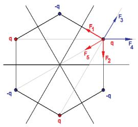
With the help of the diagram shown above, we can solve the problem. We replace the effect of the two grounded planes with five image charges at the vertices of a hexagon.
