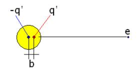
The value of  $q' = -\frac{eR}{a} = -\frac{e(1nm)}{10nm} = -e/10$  and the distance  $b = \frac{R^2}{a} = \frac{(1nm)^2}{10nm} = 0.1nm$ To find the force we subtract the repulsive force due to -q' from the attractive force of q' as follows:
