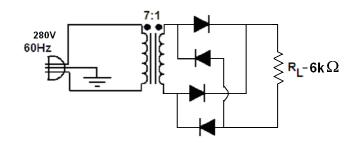
**Solution:** We recognize the circuit as a full wave rectifier in the popular configuration where the circuit forms a bridge and the current always goes through two diodes.
