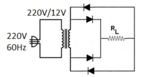
The load resistance has a value of  $R_L=0.125\Omega$  and the transformer has a nominal relation of 220V/12V, however consider possible fluctuations of +/- 8%. Specify for the diodes:
