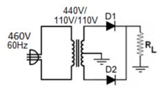
**Problem 3.-** Calculate the amplitude of the second harmonic at the output of a full wave rectifier. Give the result compared to the amplitude of the original sine wave.
