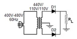
**Solution:** The worst case scenario happens when the source voltage is 480V, in this case the transformer output will be  $\frac{110}{440} \times 480 = 120V$ , with this value:
