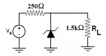
**Solution:** Consider that we increase the source voltage from zero. If the voltage in the node that connects the two resistances together is less than 4.8V, there will not be any current through the diode and the network will behave as a simple voltage divider. In this case, the voltage in the load will be
