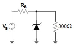
**Solution:** To maintain the voltage stable in the load it should be 5.1V even with the minimum source voltage. We can find the maximum  $R_s$  by assuming that the current in the diode is zero in this condition, so:
