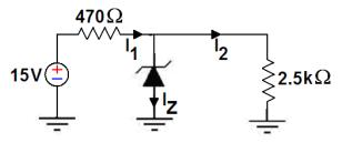
If the Zener voltage is 7.2V, the current I<sub>2</sub> will be:  $I_2 = \frac{7.2V}{2500\Omega} = 2.88mA$ . We can also calculate the current through the 470-ohm resistor:  $I_1 = \frac{15V - 7.2V}{470\Omega} = 16.60mA$ The difference between these two currents is the current through the diode:
