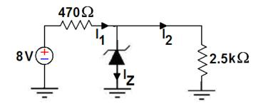
If the Zener voltage is 7.2V, the current I<sub>2</sub> will be:  $I_2 = \frac{7.2V}{2200\Omega} = 2.88mA$ , like before, and the current through the 470-ohm resistor would be:  $I_1 = \frac{8V - 7.2V}{470\Omega} = 1.7mA$
