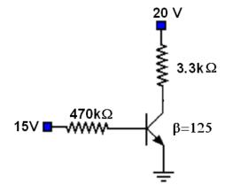
Solution: To find the Q-point of the transistor we first find the base current:
