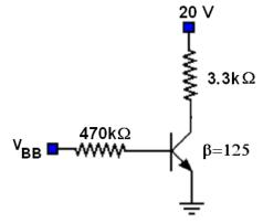
**Solution:** When the transistor is in saturation the voltage collector emitter is very low (recall from your experiments in the lab that it is typically  $\approx 0.1V$ ), so we can say that all the voltage of the power supply is across the 3.3kohm resistor, then the collector current is:
