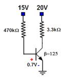
The loop equation gives us:  $15V = 470k\Omega I_B + 0.7V \rightarrow I_B = \frac{15V - 0.7V}{470k\Omega} = 30.4\mu A$ The collector current is:
