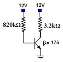
Problem 3.- Calculate the maximum value of R<sub>B</sub> that still puts the transistor in saturation.
