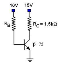
**Solution:** If the transistor is saturated, the voltage collector emitter will be very low. Let us assume it is zero, so the 15V of the source has to drop across the collector resistor:
