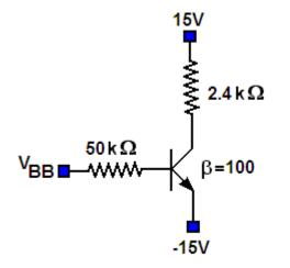
**Solution:** The voltage base-emitter has to be 0.7 or less for the transistor to be in cutoff, so  $V_{BB}$  has to be less than **-14.3** V
