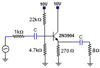
In DC the capacitors behave as open circuits and the voltage divider that feeds the base gives us the following Thevenin equivalent
