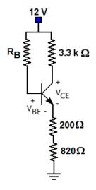
In the collector-emitter branch, we can write this equation
