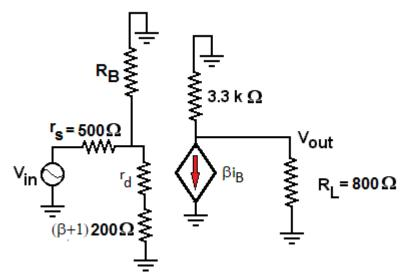
The input impedance of the amplifier is
