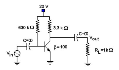
Solution.- This is a direct polarization with a fixed DC base current:
