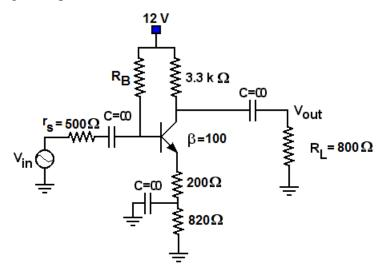
Solution: First, we do the DC analysis with the capacitors modeled as open circuits.
