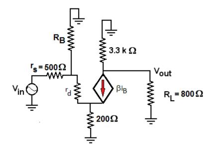
Because the capacitors behave as short-circuits in AC, the 820 $\Omega$  emitter resistance doesn't participate in the analysis, but the 200 $\Omega$  does. The current that runs through this resistance is  $(\beta + 1)$  times the base current, so it can be modeled as a  $200\Omega \times (\beta + 1)$  resistance from the point of view or the base.
