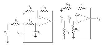
The first stage is the low pass filter and we select the components to have a cutoff frequency of 300kHz
