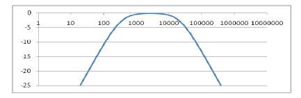
At 300 Hz the gain is 0.66 or -3.6dB
