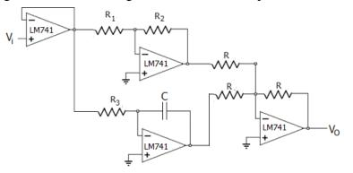
The follower at the input assures that the circuit will not load the error signal as it presents very large impedance.
