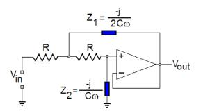
To simplify the circuit, we replace the star connection made by the two resistors and  $Z_1$  for a delta connection as follows:
