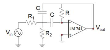
**Solution**: We can define  $X = \frac{1}{\omega C} = \frac{1}{2\pi fC}$  as the impedance of the capacitor and then the circuit using complex numbers to model the circuit:
