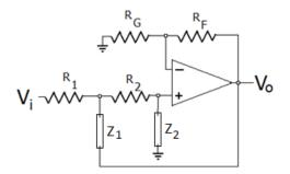
The star circuit formed by  $R_1$ ,  $R_2$  and  $Z_1$  can be converted into a delta
