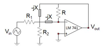
Notice that the two capacitors and the resistance R form a delta configuration, which we can transform into a star as shown below.
