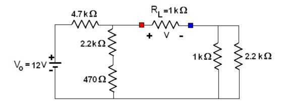
Calculate the Thevenin voltage and resistance from the point of view of the load resistance. In your calculations use the actual values of the resistors with 3 significant figures, not the nominal values.
