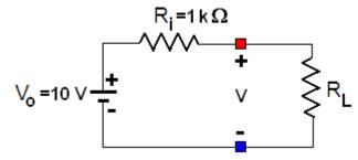
This circuit will behave like a 10mA current source with an internal resistance of 1k $\Omega$ . Calculate and measure the expected current for load resistors of 0 $\Omega$  (short circuit), 10 $\Omega$ , 47 $\Omega$ , 100 $\Omega$ , 470 $\Omega$  and 1k $\Omega$ .
