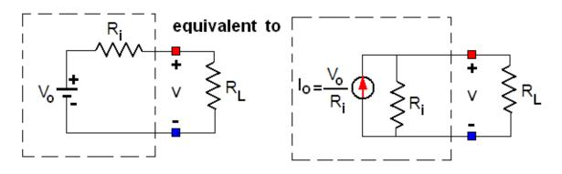
In this case, the current flowing through the load resistor can be calculated with the current divider rule. It goes like this: the ideal current is divided between the two resistors  $R_i$  and  $R_i$  inversely proportional to the values of the resistors, so:
