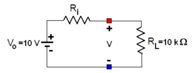
Make sure that the output of the power supply is 10V (the display in front of the P.S. is only a rough indication, use the multimeter for a more precise reading). For the internal resistor use  $10\Omega$ ,  $47\Omega$ ,  $100\Omega$ ,  $470\Omega$ ,  $1k\Omega$ ,  $4.7k\Omega$  and  $10k\Omega$ .
