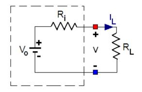
In this case the voltage at the terminals is given by:  $V = R_L I_L = V_o - R_i I_L$
