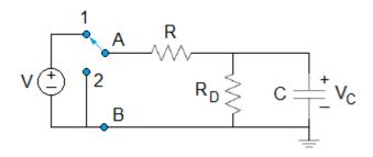
Calculate the time constant of this modified circuit. Determine the internal resistance of the DMM from your measured data.
