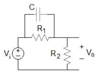
Using the supplied components, construct the circuit shown in the figure above on a breadboard. Use the values of  $R_1 = 100 \text{ k}\Omega$ ,  $R_2 = 47 \text{ k}\Omega$ ,  $C_1 = 0.1 \mu\text{F}$  or close to those values from the components available.
