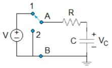
Build the circuit. CAUTION: Make sure you connect the capacitor correctly (polarity!)
