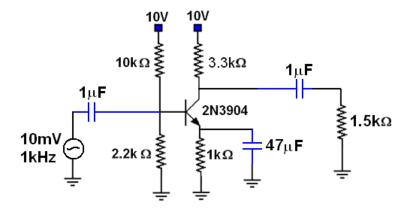
d) Calculate the voltage gain that you expect. Measure the gain using the oscilloscope. Check that the input and output signals are shifted 180°.
