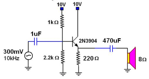
b) Calculate the voltage gain that you expect. Measure the gain using the oscilloscope.
