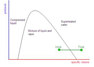
Since the process is at constant pressure, the heat is equal to the change in enthalpy. The enthalpy in the final state comes from the superheated water tables:
