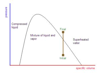
To determine the final condition of the water, we look in the superheated water tables to find the specific volume 0.1309 m<sup>3</sup>/kg at T=250°C. We find that the pressure will be between 1.6 MPa and 1.8 MPa.
