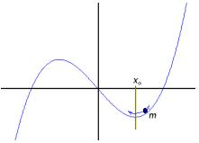
**Solution:** The potential given has a minimum when  $x = x_o = \sqrt{\frac{b}{3a}}$ , which means that it will be an equilibrium point, in other words the force will be zero there.
