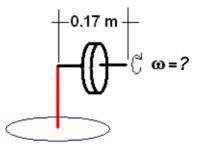
The gyroscope has an angular momentum of  $L = I\omega = \frac{1}{2}MR^2\omega$  and the torque due to its weight is:  $\tau = \frac{dL}{dt} = Mgr$ , where *r* is the distance from the center of mass to the pivot  $(r = \frac{0.17m}{2} = 0.085m$  in this problem) to complete one turn we need to cover  $2\pi L$ , so:
