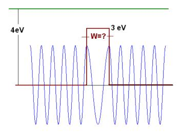
**Solution:** The condition for no reflection is:  $W = \frac{n\lambda}{2}$ , where *n* is an integer and  $\lambda$  is the de Broglie wavelength in the barrier. We also know that
