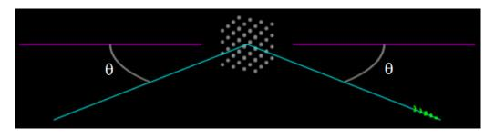
The peaks in the Bragg diffraction occur when the reflection from the planes interfere constructively, which happens when the extra distance traveled by the waves is a multiple of the wavelength according to the equation:
