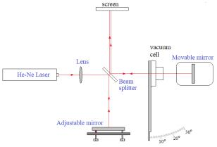
The idea is to get the number of peaks in the interference pattern as a function of gauge pressure. Once again, you should decide what the best way to do this is. Perhaps you can try with 5cm Hg, 10cm Hg and so on. It will not be possible to reach 1atm (76cm Hg) but we will extrapolate to that value once you have the data (let's call that extrapolated number of peaks n).
