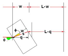
The experiment consists in turning the glass an angle  $\theta$  and counting the number of fringes that change. The change is due to the longer time it takes for light to travel in glass as compared to air. The times in the two cases are:
