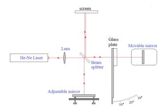
The diagram below represents the laser going through the glass plate with thickness w, then bouncing on a mirror and covering the same path again.
