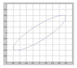
It is a case of elliptical polarization, with the ellipse rotated at an angle of 35.7°
