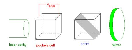
The prism has high transmission when the polarization is vertical and high reflectivity when the polarization is horizontal. The Pockels cell rotates the polarization 90° which builds energy in the laser cavity in the horizontal polarization. When the voltage is switched to zero the energy is dumped as a pulse.
