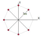
**Solution:** Consider the seven masses as a symmetric octagon minus one mass missing, so the center of mass is:
