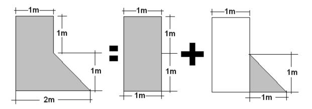
The rectangle has a mass proportional to its area:  $m_1 = (2m)(1m)\rho t$  and has a center of mass at  $x_1 = 0.5m$  and the triangle:  $m_2 = \frac{(1m)(1m)}{2}\rho t$  and center of mass  $x_2 = 1m + 0.33m$ , so the center of mass is:
