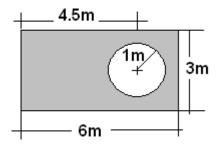
**Solution:** To solve this problem we can think of the figure as a rectangle plus a circle with negative mass. We do not know the masses, but the plate is uniform, so the masses are proportional to the areas. In fact, the mass can be calculated as area times surface density ( $\rho_s$ ). With this in mind, the table in this case is the following:
