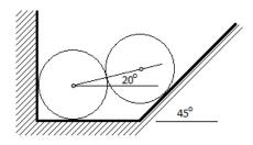
**Problem 6.-** Calculate the force in the cable if the weight of the cart is mg = 1250 N and there is no friction between the wheels and the inclined surface.
