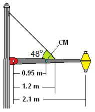
Problem 2.- Calculate the tension (force) in the cable. Neglect the weight of the pole.
