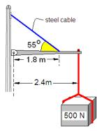
**Problem 2a.-** Calculate the horizontal force  $(F_x)$  acting on the hinge. Neglect the weight of the pole.
