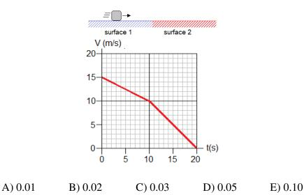
**Solution**: We notice that in the second surface the block decelerates at a rate of  $1 \text{m/s}^2$ . This indicates that the friction force is  $m(1 \text{m/s}^2)$  and since the normal force is mg, the friction coefficient is  $\mu = (1 \text{m/s}^2)/(10 \text{m/s}^2) = 0.1$ Answer: **E**  **Problem 3.-** In the following cases there is no friction, and the force F is the same. Analyze in which case the tension of the string between the masses is maximum.
