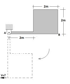
**Problem 5a.**- Consider a mechanical piece in the shape of an L, built by joining two identical thin 20cm long bars AB and BC. The piece is released from rest from the position shown below and it rotates freely around A. Calculate the velocity of point B when it passes the vertical line below A.
