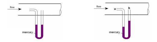
**Problem 7a.-** A Pitot tube is an instrument used to measure airspeed of an aircraft or fluid flow in pipes. In the following schematic, the mercury is leveled because there is no airflow. When the flow starts, the level on the right goes up 0.5mm (and the level on the left goes down 0.5 mm). Calculate the speed of the air if the density of air is 1.29kg/m<sup>3</sup> and the density of mercury is 13,600 kg/m<sup>3</sup>.
