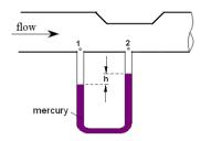
**Problem 5b.-** The Venturi tube shown in the figure has a restriction in the cross section, so the speed of the air flow at point "2" is 15 m/s, while the speed at point "1" is 10 m/s.
