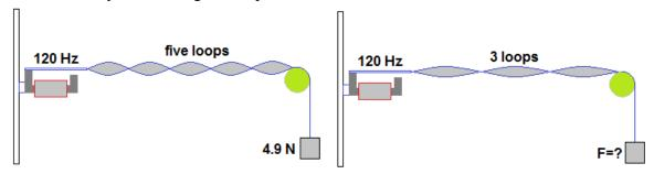
**Solution:** Notice that in the equation  $f = \frac{n}{2L} \sqrt{\frac{F}{\rho_{linear}}}$  the force is inversely proportional to the
