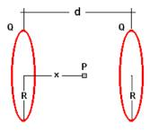
**Problem 7.-** Find the point P on the x-axis on the right side of the positive charge where the electric potential is zero:
