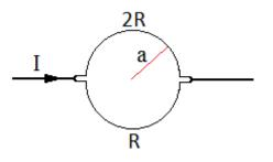
**Solution**: Since the resistance at the top is higher, the current will be lower. We can use Ohm's law to calculate the currents. If we call them  $I_1$  and  $I_2$  as indicated:
