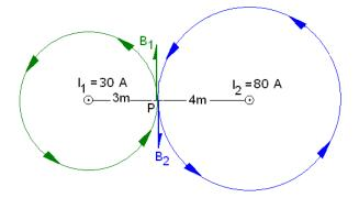
The sum of the two vectors is  $2\mu T$ , downward direction.
