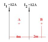
**Solution:** The magnetic field at point A is **zero**. At point B there are two contributions:
