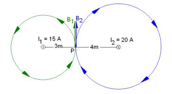
The sum of the two vectors is  $2\mu T$ , upward direction.
