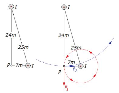
Magnetic field produced by a long wire:  $B = \frac{\mu_o I}{2\pi r}$ , where  $\mu_o = 4\pi \times 10^{-7}$ For the wire that is 24 meters away:  $B_1 = \frac{\mu_o I}{2\pi r} = \frac{4\pi \times 10^{-7} \times 150}{4\pi \times 24} = 1.25 \,\mu\text{T}$
