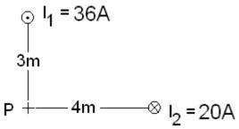
Solution: Each wire produces a magnetic field at point P as follows:
