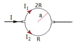
Ohm's law means that  $2RI_1 = RI_2$ , which means that  $I_1$  is half  $I_2$ . And the sum is I, so the currents are  $I_1 = I/3$  and  $I_2 = 2I/3$ .
