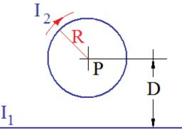
**Solution**: The direction of  $I_2$  is such that at P it produces a magnetic field towards the figure. The current  $I_1$  must flow to the right to counteract  $I_2$ . We equal the two magnitudes to get zero.
