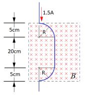
**Problem 11.-** Calculate the net force on the conductor, due to the magnetic field B = 0.25 T shown in the figure.
