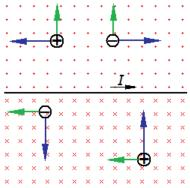
**Problem 6.-** The particle shown in the figure enters a region of magnetic field and is deflected upward. Is the charge of the particle positive or negative? Explain.
