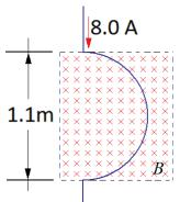
**Solution**: To calculate the force we divide the semicircle in small segments of arc *dl* as shown in the figure.
