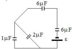
The  $1\mu$ F and  $2\mu$ F capacitors in the circuit are also in parallel as their terminals are connected to the same voltage. It does not matter that they do not appear physically in parallel as one is vertical and the other diagonal.
