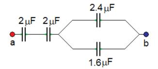
This  $2.4\mu$ F is in parallel with a  $1.6\mu$ F capacitor. They are equivalent to:
