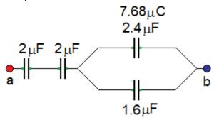
This charge is the same for the two capacitors in series that make up the equivalent. So going back one step to the original circuit we get:
