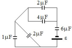
The charge in that capacitor is zero.
