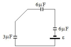
Finally, the three capacitors in this last circuit are in series, so they are equivalent to
