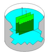
**Problem 2a.-** If it weren't for practical reasons that prevent it, water would be a good choice to make capacitors since its dielectric constant is very large ( $K_{water}$ =81). Calculate the capacitance (in farads) of two plates submerged in water if their area is 0.25 m<sup>2</sup> and the distance between them is 0.55 mm.
