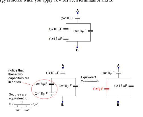
Now, notice that the  $9\mu$ F capacitor is in parallel with the  $18\mu$ F one, so they together are equivalent to  $18\mu$ F +  $9\mu$ F = 27  $\mu$ F. Giving the circuit shown in the figure below:
