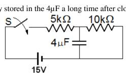
**Solution**: In DC circuits capacitors behave like open circuits after a long time. The current in the resistors after a long time will be  $15V/15k\Omega = 1$ mA. The voltage in the  $10k\Omega$  resistor will then be 10V, which is also the voltage in the capacitor. Then the energy will be
