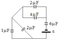
The charge in that capacitor is zero.
