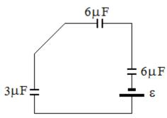
Finally, the three capacitors in this last circuit are in series, so they are equivalent to
