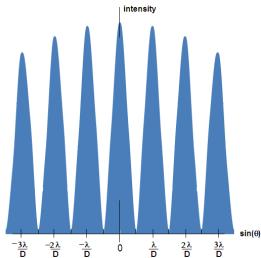
There is a maximum in intensity anytime the sine of the angle is an integer times the wavelength over the distance between the slits. The effect of the slits' width is an overall pattern like the one for a single slit (not shown above).
