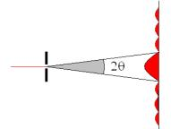
**Problem 1a.-** A thin rectangular aperture is illuminated with a He-Ne laser (like you did in the lab) and it is observed that the first dark fringe happens at an angle of 3.55° from the center. Calculate the width of the aperture knowing that the wavelength of the laser is 632.8 nm.
