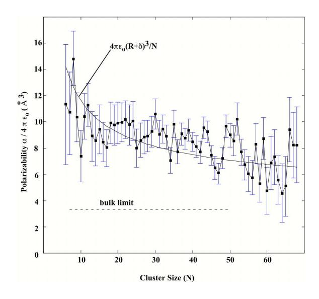
Figure 41: Polarizability per atom of vanadium clusters measured at 300 K and 72 kV/cm. The dashed line is the bulk limit and also shown is the polarizability calculated with the spill-out approximation (equation 6) for  $\delta$ =0.18 nm
